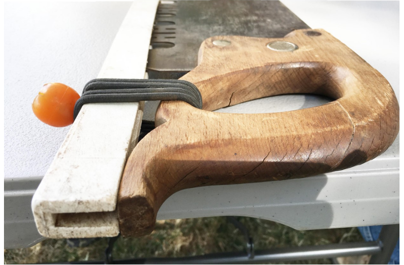
Securely-tied guard for saw teeth; ready for mule packing
